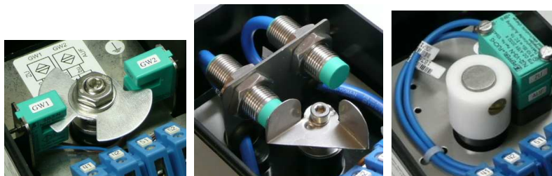
Image 3-5: Pepperl+Fuchs sensors 2x SJ 3,5-N, 2x NJ2-12GK-N and 2x NJ2-V3-N
