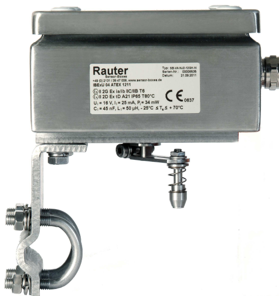
Image 13: Stainless steel limit switch box, 150x150x80mm, IP 65, - 25 °C up to + 70 °C, for linear actuators acc. to Namur IEC 534 with mounting set
