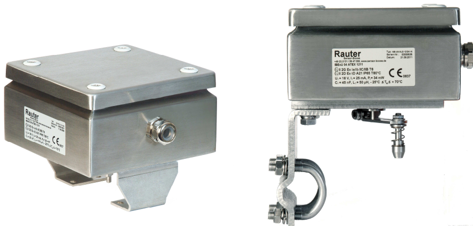
Image 1-2: Stainless steel limit switch boxes, A2, IP 65, 150x150x80mm with F05-slot, left: for rotary actuators acc. to VDI/VDE 3845 with bracket, right: with mounting set for linear actuators acc. to NAMUR IEC 534
