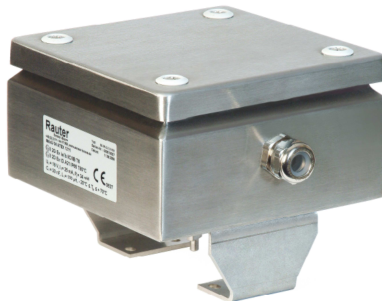
Image 12: Stainless steel limit switch box, 150x150x80mm, IP 65, - 25 °C up to + 70 °C, for rotary actuators acc. to VDI/VDE 3845 with bracket
