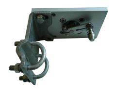
**images:** Mountable at cast-,flat- and pillars valve yokes: Stroke: 10 up to 35 and up to 100mm, the aluminium plate is not included in the set.
