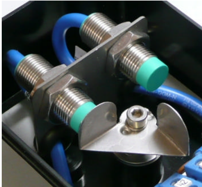
image: inner view Pepperl+Fuchs sensors NJ-12GK-N with 0 and 90° switching cam
