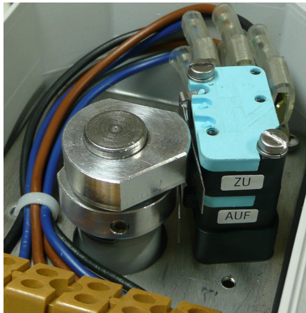
image: inner view Crouzet limit switches with adjustable switching cams
