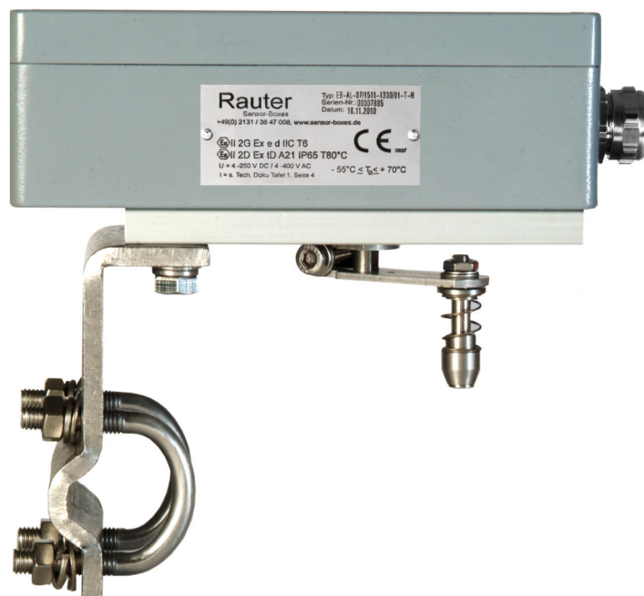
Image 10: Low temperature limit switch box, aluminium housing, 175x80x57mm, for linear actuators, -55°C ≤ T a ≤ +70°C, 175x80x57mm, IP 65, inner view see image 9
