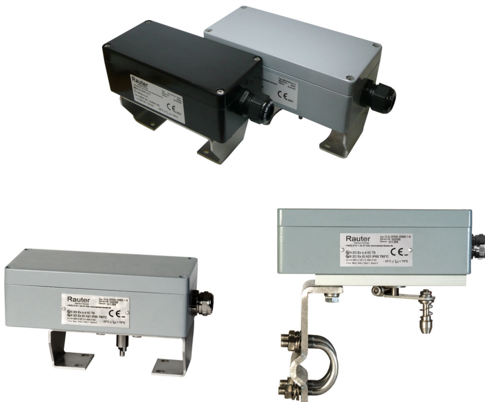
Image 1-3: Polyester and aluminium limit switch boxes for rotary actuators, -20^{\circ}\text{C} \leq T_a \leq +70^{\circ}\text{C} , 160x75x55mm/175x80x57mm, IP 65, low temperature limit switch boxes for rotary and linear actuators, -55^{\circ}\text{C} \leq T_a \leq +70^{\circ}\text{C} , 175x80x57mm, IP 65
