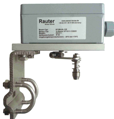
image 3: limit switch box, aluminium housing for linear actuators with mounting set acc. to NAMUR IEC 534, size: 125x80x57mm
