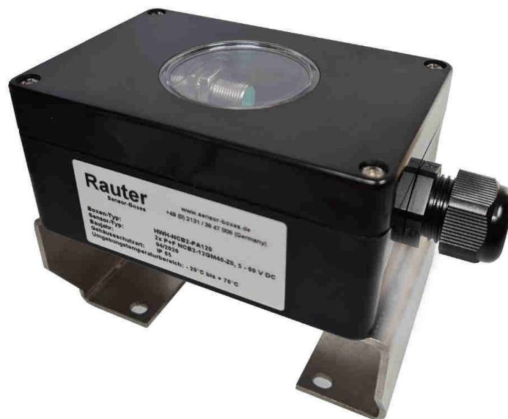
Image 1: Polyamide (Vestamide) limit switch box, 120x80x55mm for actuators acc. to VDI/VDE 3845 with 20mm stem height and hole spacing 80x30mm.
