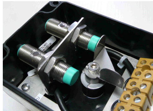
Image 2+3: Inner view 24 V DC Pepperl+Fuchs sensors, left 2x SB 3,5-E2 with 2x aluminium adjustable switching cams for position open/closed (0° - 180°), right 2x NJ2-12GM40-E2 with stainless steel switching cam for position open/closed, 0° and 90°, connecting on 6-pole clamp
