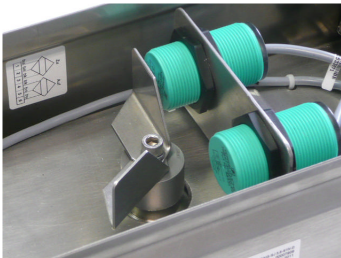
Pepperl+Fuchs limit switches NBB10-30GK50-E2 and adjustable switching cam
