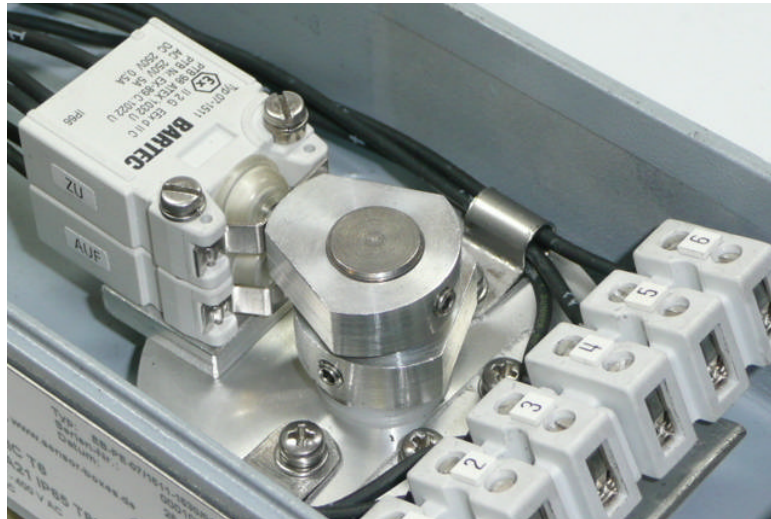
image: inner view Bartec - 55°C limit switches 07/1511-1330/01 with adjustable switching cams
